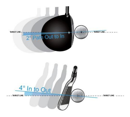
To hit the ball straight, the clubhead path should be zero. The clubhead path affects the curvature of the ball's flight trajectory and its launch direction.
