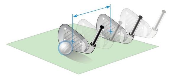
Clubhead speed indicates a player's potential distance, but distance is significantly impacted by factors such as impact point, attack angle, clubhead trajectory, and the angle of the clubface relative to the swing path. Ball speed and clubhead speed form an interesting relationship. Insufficient clubhead speed can be caused by poor weight transfer, insufficient pelvic and chest rotation, poor force sequencing, and a lack of speed training.
