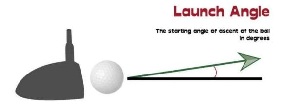
Launch angle affects the height and landing distance of the ball's trajectory. Most golfers initially believe that launch angle is closely related to the angle of attack, but in reality, depending on the shot type and clubhead speed, the angle of attack contributes between 17% and 37% to the launch angle. The largest contributor to the launch angle is the dynamic loft at impact, which contributes between 63% and 83%.
