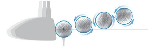
Spin has a significant impact on the lift and drag generated by a golf ball during flight, affecting its flight distance, altitude, trajectory curvature, and roll after landing.
